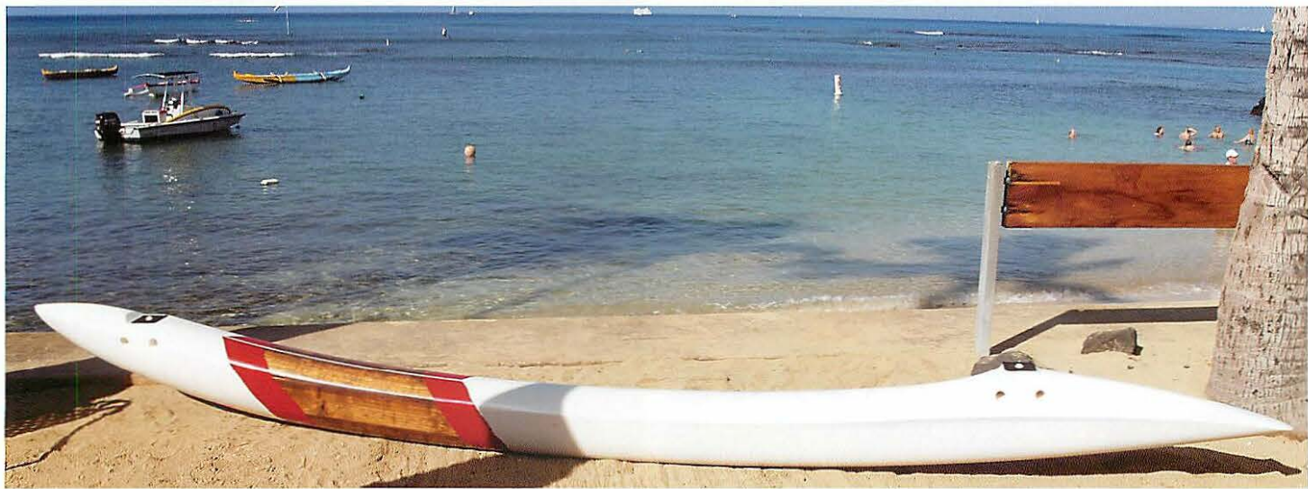
The ama for the Kaoloa is molded from koa and fiberglass.
